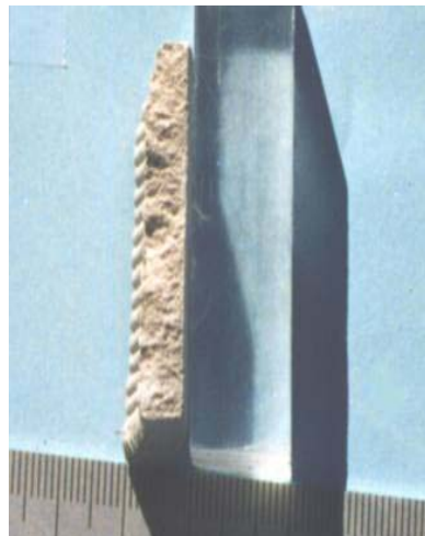
Figure 5-11. The cross section profile of a clay part
