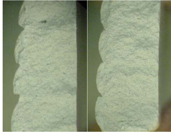
Figure 7-9. Cross section of the fabricated parts by (a) an elliptical, and (b) a square orifice
