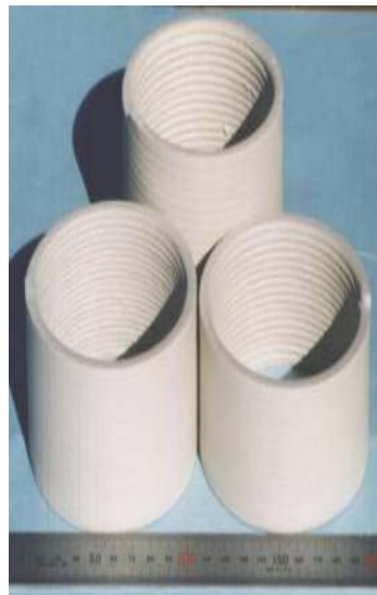
Figure 5-13. The clay parts showing superior surface finishes with consistent thickness
