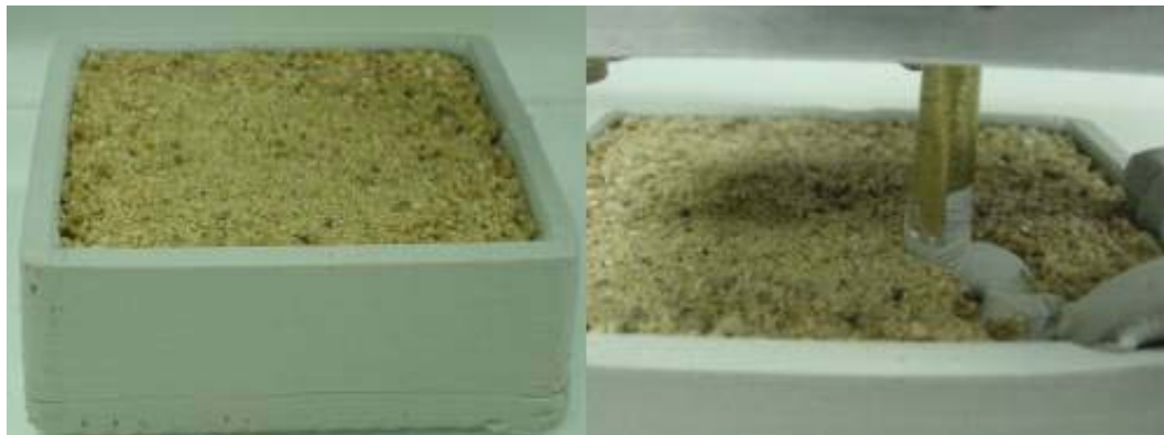
Figure VII-3. Effect of sand: (a) after part being filled with the sand, and (b) during the fabrication of the second part
