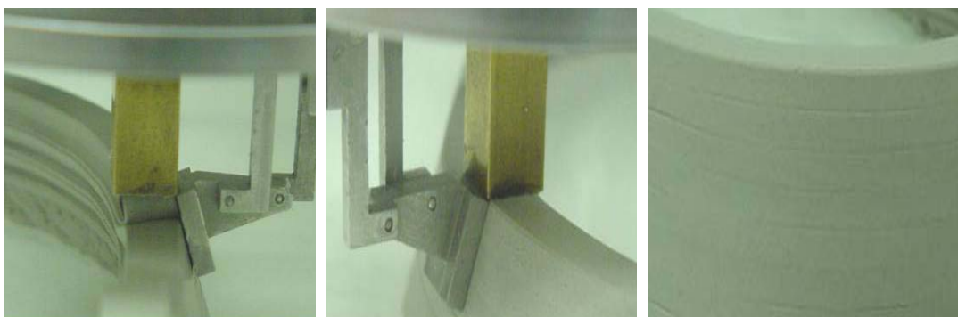
Figure 7-23. On-line process with two side trowels: (a) front view, (b) back side view, and (c) surface quality
