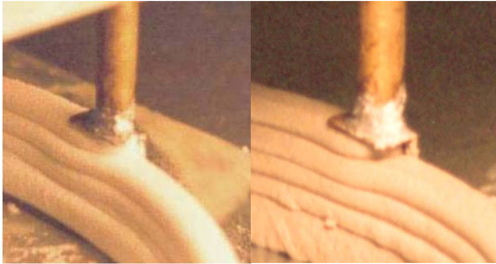
Figure 5-10. Compression and spring-back during fabrication; a) with plaster, and b) with clay
