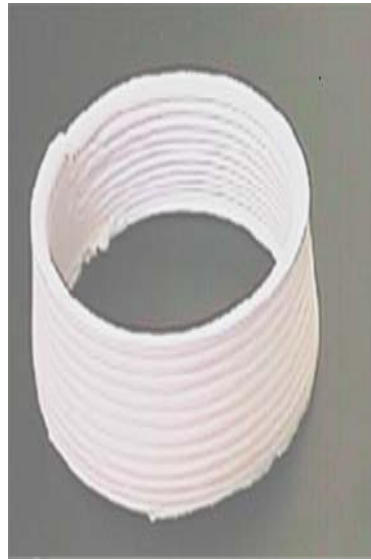
Figure 5-5. Plaster part extruded without heating and wetting
