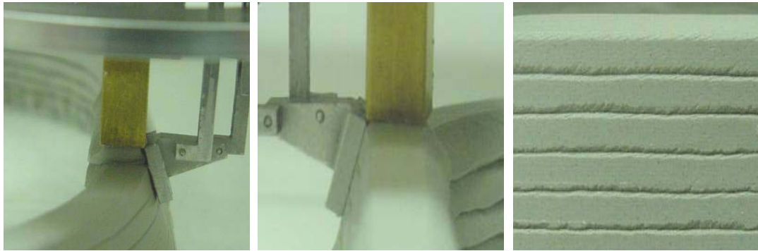
Figure 7-21. On-line process with an exterior angle: (a) front view, (b) back side view, and (c) surface quality
