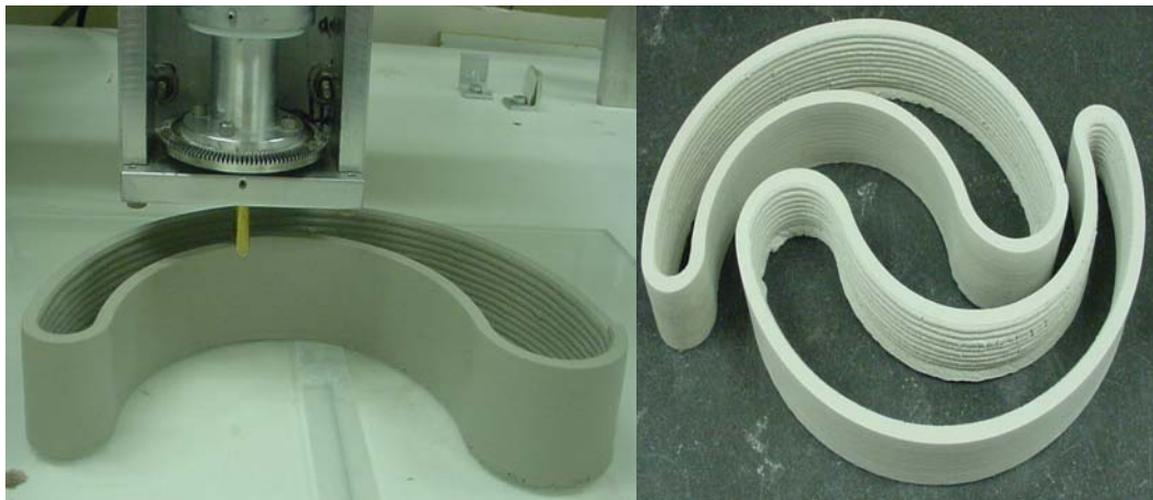
Figure III-2. Complicated profile similar to that of a turbine blade being made using CC
