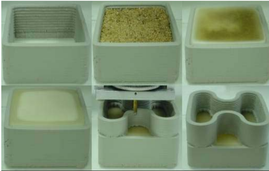
Figure VII-4. Process steps: (a) Fabricate the first part, (b) Fill the sand into the first part, (c) Coat its top surface with wax, (d) Wetting the top surface of the topmost layer, (e) Fabricating the second part on it, and (f) Completing the second part
