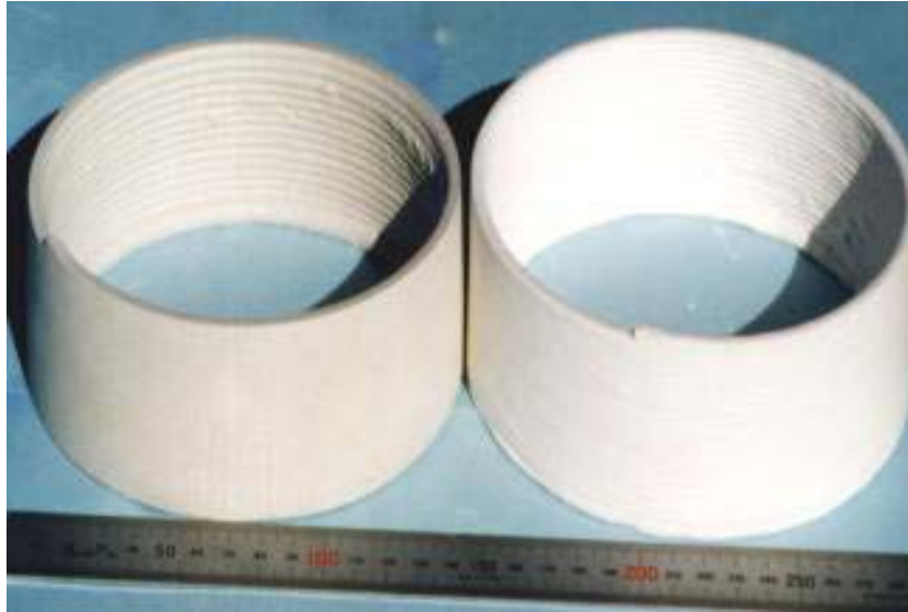
Figure 5-12. The parts showing adequate surface finish with different materials used
