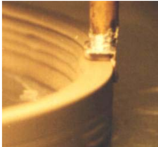
Figure 7-1. Clay part showing compression and spring-back during fabrication from the front view
