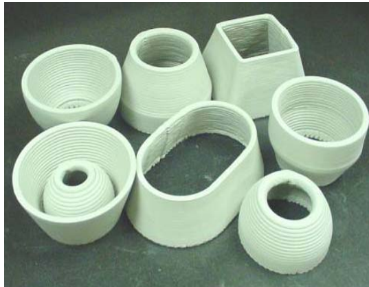
Figure 6-25. Various primitive geometries fabricated with the pivoting side trowel
