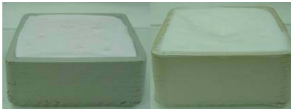
Figure VII-2. Effect of a paste: (a) after part being filled with the soft paste, and (b) after the part is solidified
